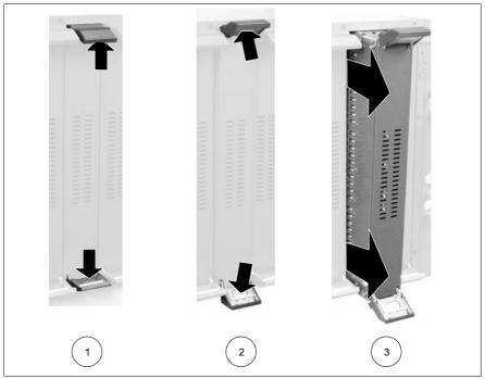
Figure 30: Removing a server blade dummy module
